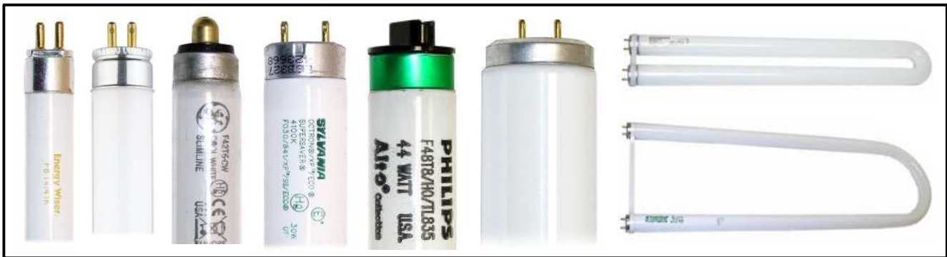
Figure 4.1: An Assortment of Linear fluorescent tubes. From left to right: T4 bi-pin, T5 bi-pin, T6, T8 bi-pin, T8 recessed contact (R17d), T12, T8 U-tubes.
