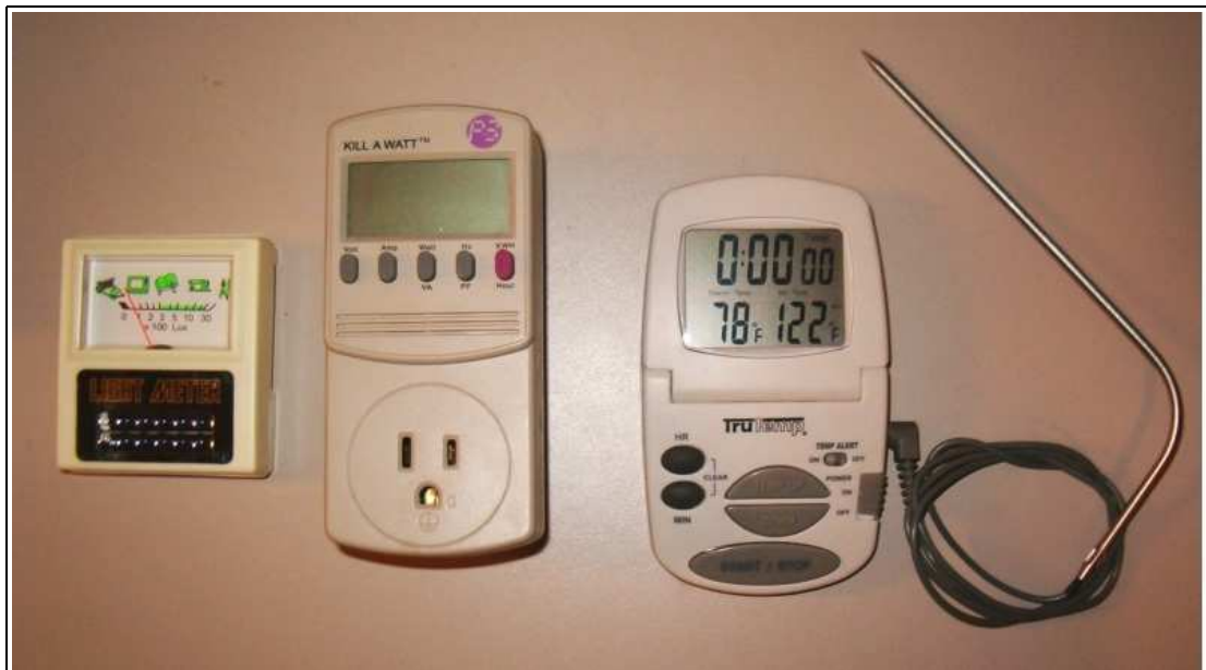
Figure 9.1: From left to right: Sight Saver™ light meter, Kill A Watt™ digital combination meter, TruTemp® digital thermometer and timer.
