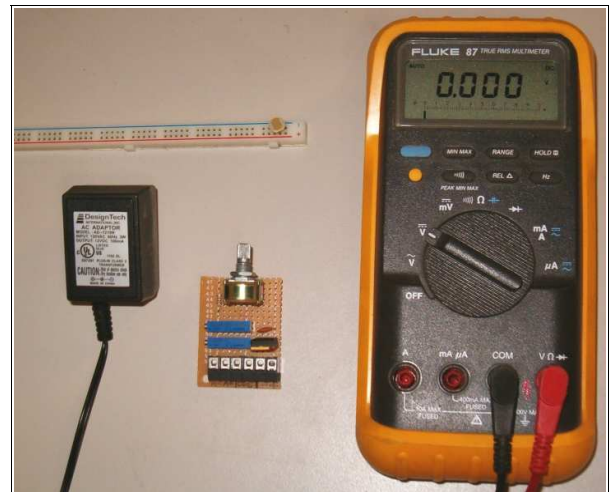
Figure 18.2 (right) All components of the light meter: AC-DC converter, CdS cell, main circuit board, digital voltmeter.
