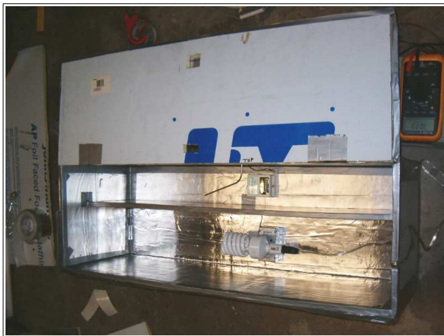
Figure 17.3 Light box with attached lid, prepared to run a test on a CFL.
