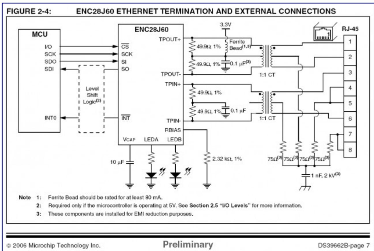
Using the application examples from both [Microchip’s ENC28J60 Datasheet](#) as well as [Guido Socher’s](#) documentation of his [AVR microcontroller based Ethernet Device](#), I have completed the preliminary schematic and parts list for my NIC sub-module. My schematic and parts lists are included below.
