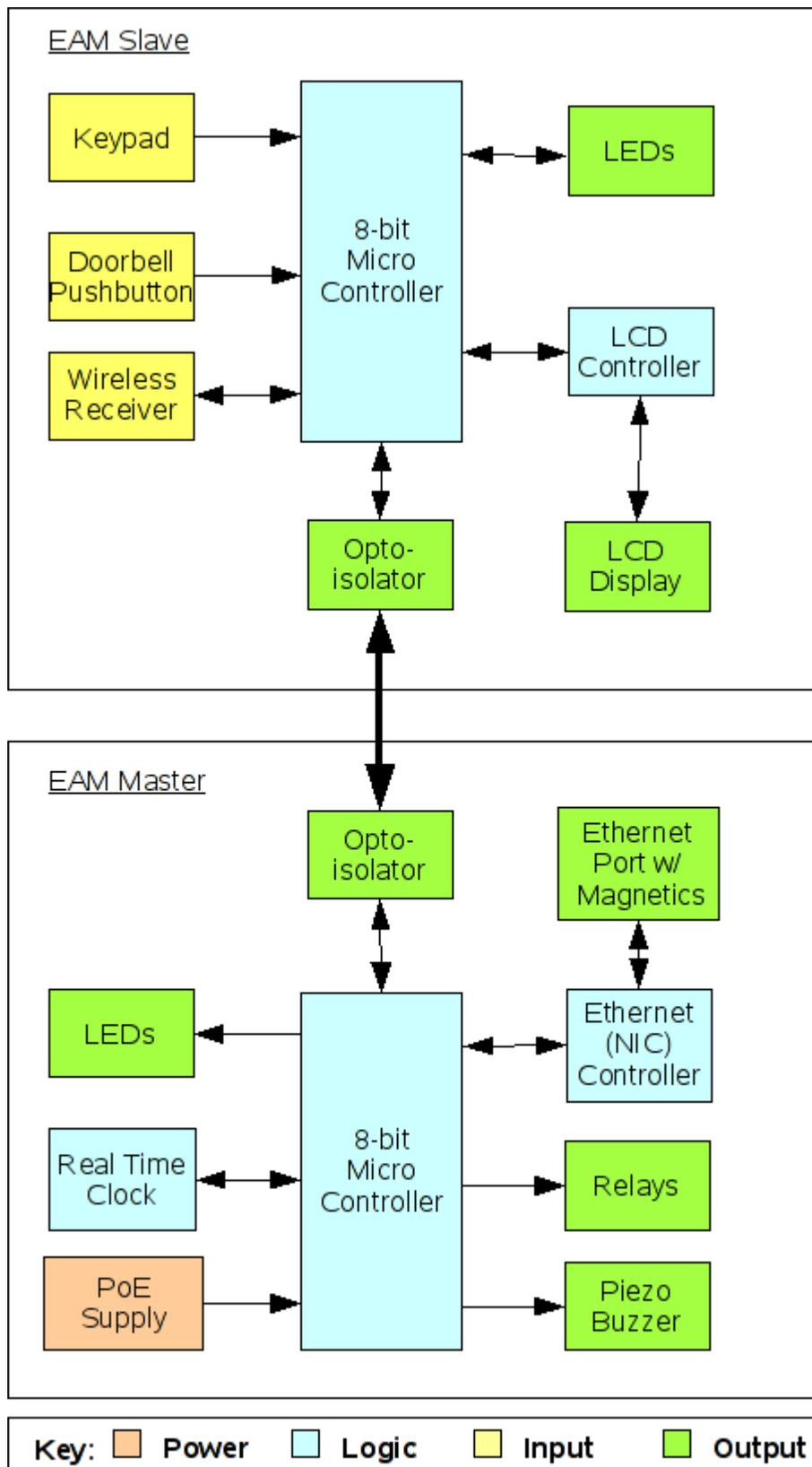
Figure 3-1: EAM Hardware Block Diagram
