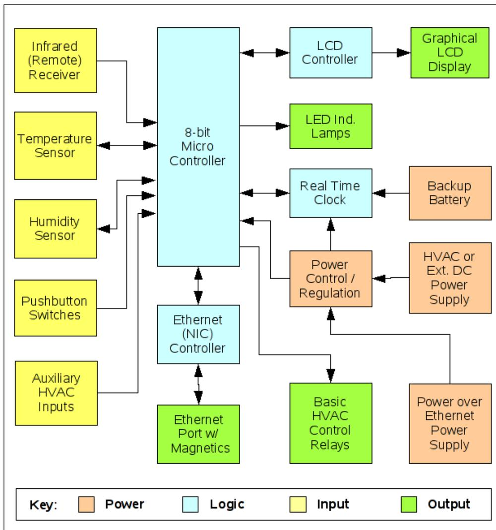
Figure 2-1: COPTA Hardware Block Diagram
