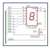
I was at first overwhelmed with the idea of controlling 70 LEDs. My initial scheme would use up 17 precious I/O pins ((1 per cathode x 10 displays) + (1 per LED x 7 segments)). This is undesirable for obvious reasons.
