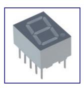
My original plan was for the EAM slave module to have an LCD or VFD screen for the passcode digit display. I'm now in favor of using individual seven segment LED displays instead for the following reasons:
